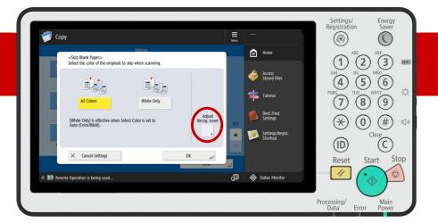
Use the [+] and [-] buttons to adjust the sensitivity. Press [OK]
